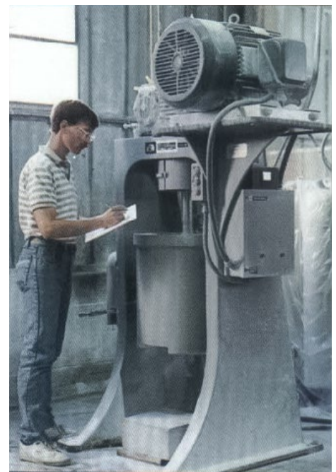
Attritor stirred ball mill is a product of Union Process, Inc., Akron, OH
