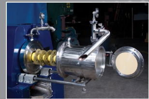
Rail system allows for easy maintenance and tank removal.
